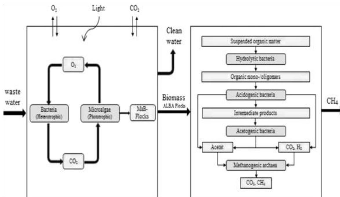
**Figure 3:** Microalga-bacterial wastewater treatment and the biogas production process
