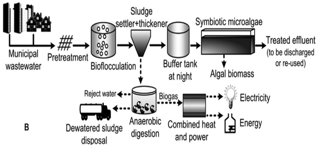
**Figure 1:** Schematic representation of a municipal wastewater treatment plant
