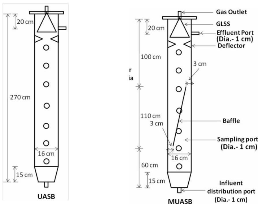
**Figure 5:** Schematic representation of UASB and MUASB reactors
