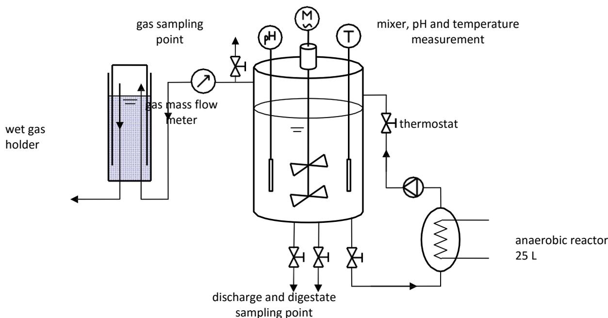
**Figure 2:** Schematic representation of an anaerobic digestion pilot plant as used in the laboratory
