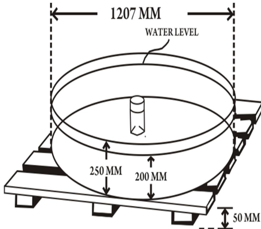
**Figure 1:** Dimensions for Class A Evaporation pan
