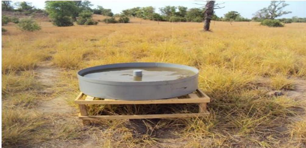
Figure 2: Installed Class A Evaporation pan at Dam Site
