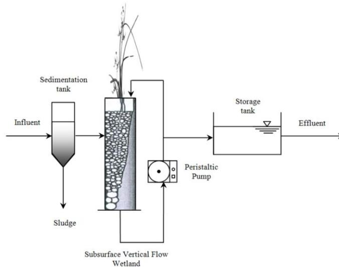
Figure 4. Combined model of sand filter and wetland
