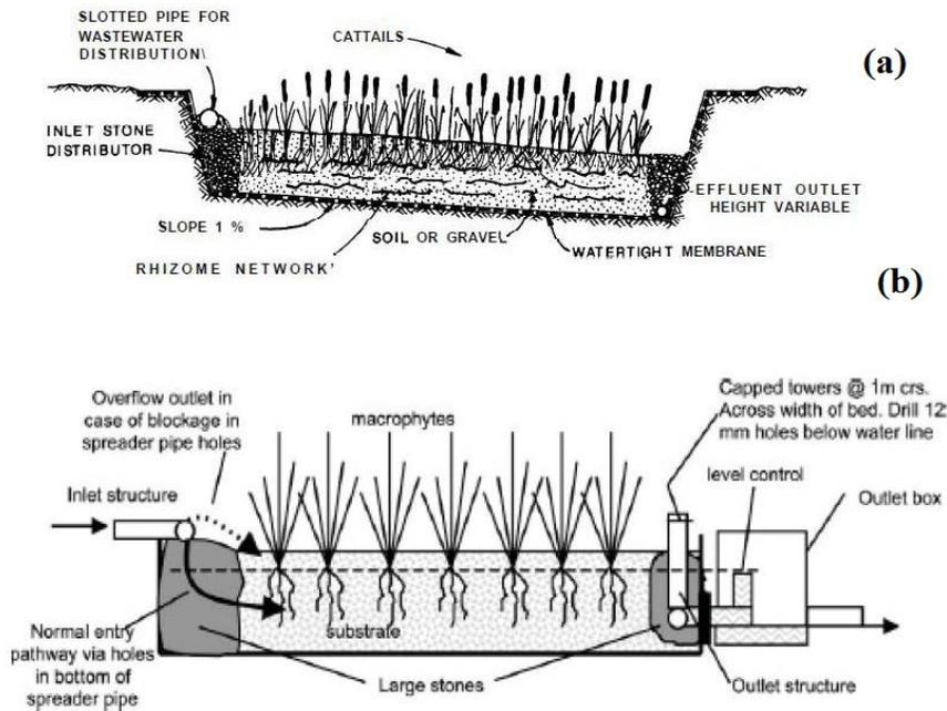
Figure 2. Types of constructed Wetland (a) Free water surface (b) Subsurface
