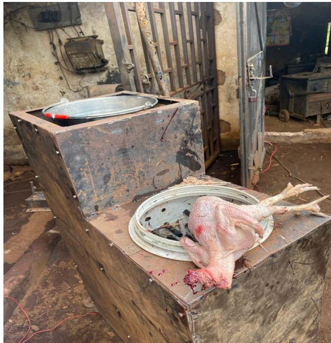
Figure 1: Poultry De-Feathering Machine (before painting) and a De-Feathered Cockerel
