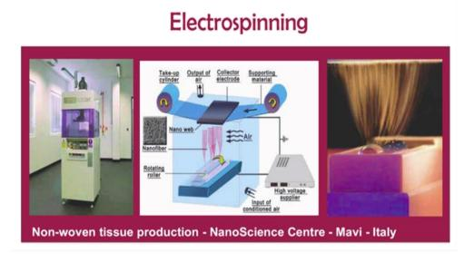
Figure 2: Electrospinning technology
