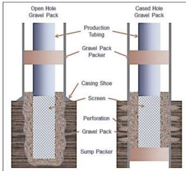
Figure 1: Internal Gravel Packing [13]
