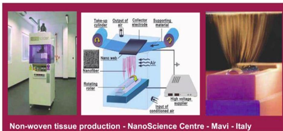
**Figure 2:** Electrospinning technology
